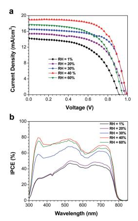
Fig. 4 (a) J-V curves of the highest performance devices measured at a scan rate of 0.83 V s<sup>-1</sup>. (b) IPCE spectra of the same devices.
