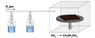
Fig. 1 Schematic of the apparatus used to control the RH inside an atmospheric bag containing a spin coater. Pbl<sub>2</sub> films are converted into CH<sub>3</sub>NH<sub>3</sub>Pbl<sub>3</sub> by immersion in a solution of CH<sub>3</sub>NH<sub>3</sub>I, spin dried at 3000 rpm for 30 s, and allowed to dry for a further 10 min.
