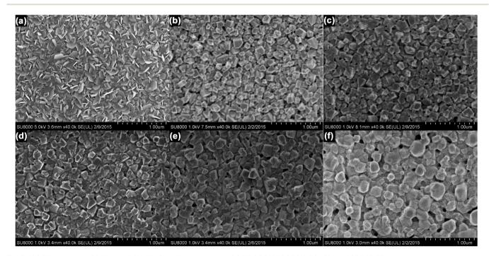
Fig. 3 (a) SEM images of (a) PbI<sub>2</sub>, and CH<sub>3</sub>NH<sub>3</sub>PbI<sub>3</sub> films prepared at (b) 1%, (c) 20%, (d) 30%, (e) 40%, and (f) 60% RH
