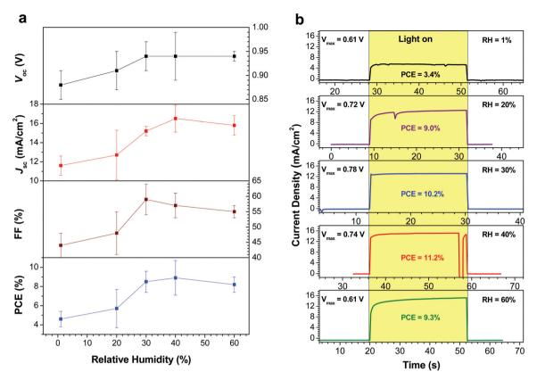
Fig. 6 (a) Average device performance characteristics (measured at a scan rate of  $0.1 \, \mathrm{V \, s^{-1}}$ ) as a function of relative humidity. Error bars represent plus or minus one standard deviation from the mean. (b) Steady-state current densities for representative devices at each relative humidity.
