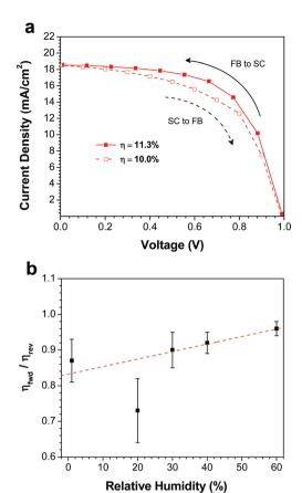
Fig. 5 (a) J-V curves measured at  $0.1\,\mathrm{V}\,\mathrm{s}^{-1}$  for the best device prepared at 40% RH. (b) Ratio of PCEs determined from forward (SC-FB) and reverse (SC-FB) scans as a function of RH. The linear fit is a guide to the eye.
