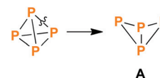
Scheme 1 Breaking one of the PP bonds in tetrahedral P 4 formally yields the tetraphosphabicyclo[1.1.0]butane scaffold ( A ).
