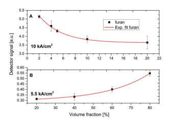
Fig. 6 riQCL-iHWG sensor system response to furan (in 2-methoxyethanol) obtained via selective emission line damping at an applied voltage of 10 kA cm $^{-2}$  (A), and of 5.5 kA cm $^{-2}$  (B). An exponential fit was applied to the response function resulting in a calibration model with a coefficient of determination  $(R^2) > 0.99$  for both curves.
