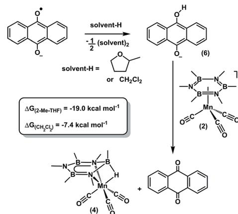
Scheme 6 Proposed net reaction, and calculated free energy, for formation of 2 via AQ mediated H-atom transfer in 2-MeTHF and CH<sub>2</sub>Cl<sub>2</sub>.
