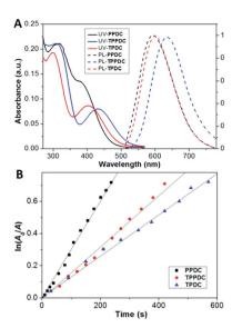
Fig. 3 (A) UV-vis absorption (solid lines) and normalized photo-luminescence (PL) spectra (dashed lines) of 10  $\mu$ M each of PPDC, TPDC and TPPDC in DMSO/water (v/v = 1/99). (B) The decomposition rates of ABDA by PPDC, TPDC and TPPDC;  $A_0$  and A are the absorbance of ABDA in the presence of the AIEgen PSs at 378 nm before and after irradiation, respectively.
