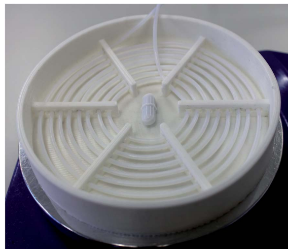
Fig. 3 Photograph of a 3D-printed oil bath with integrated mounting holes for holding PTFE tubing in a fixed spiral arrangement.
