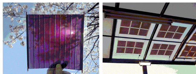
Fig. 1 (Left) P3HT-based OSCs on a flexible substrate. (Right) Evaluation of long-term stability of OSCs on the top of roof. Reproduced with the permission from ideal star inc.
