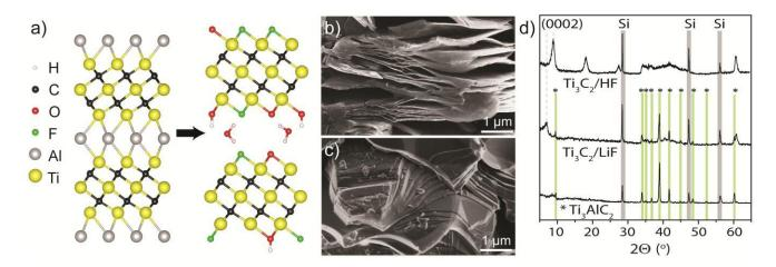
Figure 1: a) Schematic of etching from  $Ti_3AlC_2$  to  $Ti_3C_2T_x$  showing terminations and interlayer water. Typical SEM micrographs of (b) HF-etched  $Ti_3C_2T_x$ , showing accordion-like structure and (b) LiF-HCl etched  $Ti_3C_2T_x$ , with a more compact structure. d) XRD patterns of  $Ti_3AlC_2$  and  $Ti_3C_2T_x$  etched with HF or LiF-HCl. Green vertical lines denote the presence of MAX phase peaks, and grey regions are peaks from crystalline Si 10 wt % internal standard.
