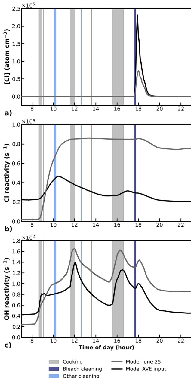
Fig. 5 Modelled Cl atom concentration (panel a, atom per cm<sup>3</sup>), Cl atom reactivity (panel b, s<sup>-1</sup>), and OH radical reactivity (panel c, s<sup>-1</sup>) for the June 25 scenario (grey) and the averaged-day scenario (black). The shaded areas on each panel indicate the timing of the indoor activities carried out during the day: cooking (grey), Cl-cleaning (dark blue), and other cleaning (light blue) activities.
