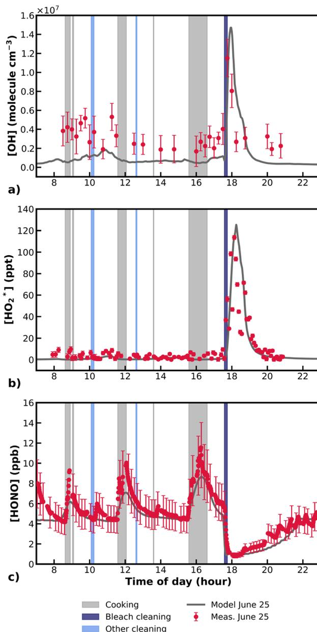
Fig. 2 Modelled (grey line) *versus* measured (red circles) concentrations of OH radicals (panel a, molecule per cm<sup>3</sup>), HO<sub>2</sub><sup>\*</sup> radicals (panel b, ppt), and HONO (panel c, ppb) on June 25. Error bars represent the experimental uncertainties. The shaded areas indicate the timing of the activities carried out during the day: cooking (grey), Cl-cleaning (dark blue), and other cleaning (light blue) activities.
