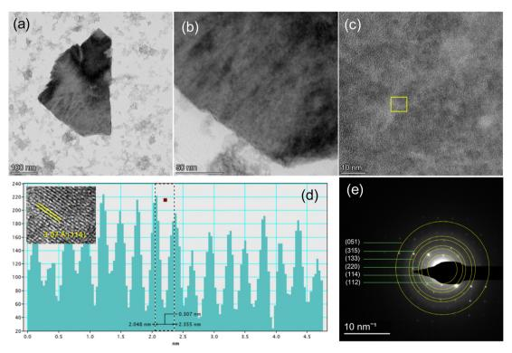
Fig. 3 (a) and (b) TEM images of Ni-doped Bi<sub>3</sub>O<sub>4</sub>Br, (c) HR-TEM image, and (d) line-scanning intensity profile of the inserted inverse FFT and live FFT of the selected area in (c). (g) SAED pattern of Ni-doped Bi<sub>3</sub>O<sub>4</sub>Br, (FFT = fast Fourier transition).
