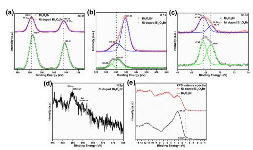
Fig. 2 High resolution XPS spectra of (a) Bi 4f, (b) O 1s, (c) Br 3d, (d) Ni 2p, and (e) valence spectra for Bi<sub>3</sub>O<sub>4</sub>Br and Ni-doped Bi<sub>3</sub>O<sub>4</sub>Br.
