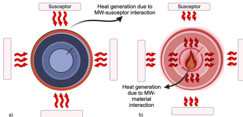
Fig. 2 A susceptor external to the sample heats a material from its surface due to the MW excitation (a), while when there is an interaction between the materials and MW, the material is heated from the centre (b). The susceptor-assisted microwave heating, supporting the material heating (b) is generally defined as “hybrid heating”.
