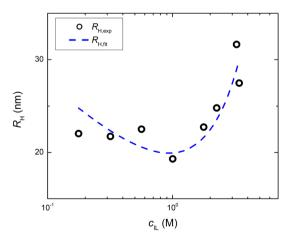
Fig. 34 Variation of the apparent hydrodynamic radius of PC<sub>4</sub>-TFSI in DMF solution at c = 0.01 M as a function of added ionic liquid (Bmim-TFSI) concentration  $c_{\rm IL}$ . The line is calculated assuming  $R_{\rm H} \propto r_{\rm scr}^{-0.4}$ , leaving the proportionality constant as a free parameter. The data are taken from
