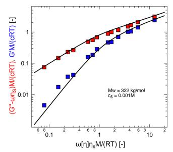
Fig. 6 Storage and loss modulus for sodium polystyrene sulfonate in 0.001 M NaCl salt solutions. Measurements at T = 5, 15, and 25 °C were plotted into a single master-curve. Lines are the Zimm model using egn (8.67) and (8.68) from ref. 86 with  $\nu$  = 0.59. Data are from ref. 274.
