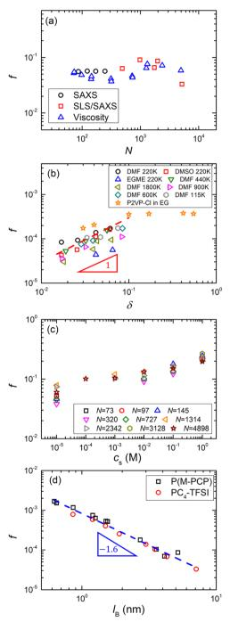
Fig. 13 The dependence of the charge fraction f on (a) the degree of polymerisation N for NaPSS, (b) the fraction of ionic monomers  $\delta$ , (c) the molar concentration of salts  $c_{s'}$  and (d) the Bjerrum length  $l_{\rm B}$ .  $c^{\star}$  data used to calculate f for plots (a)-(c) are from Fig. 11. Plot (d) uses  $c^*$  data from
