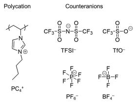
Fig. 1 Representative chemical structures of a PIL polycation and four different types of counteranions. Polycation:  $PC_4^+$ ; poly(1-butyl-3-vinylimidazolium), counteranions: TFSI<sup>-</sup>; bis(trifluoromethanesulfonyl)imide, TfO<sup>-</sup>; trifluoromethanesulfonate,  $PF_6^-$ ; hexafluorophosphate,  $BF_4^-$ ; tetrafluoroborate.
