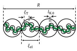
Fig. 2 Dilute polyelectrolyte chain adopts an extended configuration of electrostatic blobs of length  $\xi_{\rm el}$  inside which the conformation is a selfavoiding walk of thermal blobs with length  $\xi_{\rm T}$ . A random walk of Kuhn segments with length  $l_{K,0}$  forms the thermal blob.
