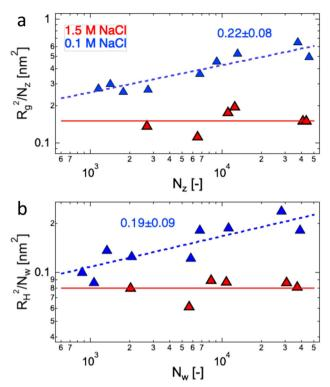
**Fig. 21** Square of (a) radius of gyration and (b) hydrodynamic radius normalised by degree of polymerisation for sodium polyacrylate at the theta salt condition (1.5 M NaCl) and below the theta salt condition (0.1 M), corresponding to the 'good solvent' universality class (expected exponent of 0.18). Errors in exponents are two standard deviations. Data are from ref. 499.
