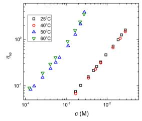
Fig. 15 Temperature induced transition for P(M-PCP) in NMF solution. Specific viscosity  $\eta_{sp}$  is plotted as a function of monomer concentration cfor P(M-PCP) in NMF at different temperatures, as indicated in the legends. Data are from ref. 174.
