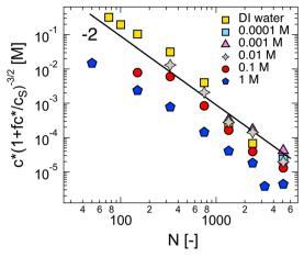
Fig. 16 Overlap concentration of NaPSS in aqueous NaCl solutions, normalised according to eqn (13). Line is power-law of -2.  $c^*$  are calculated using  $\eta_{\rm sp}(c^*)=1$  criterion using data from ref. 100. A residual salt content of  $c_{\rm s}=7.4\times10^{-5}$  M was assumed. 100
