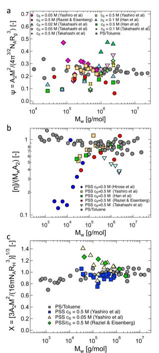
Fig. 28 Comparison of the universal ratios  $U_{nA}$  (a),  $\Psi$  (b) and X (c) for polystyrene in good solvent (grey symbols) and NaPSS in aqueous salt solutions (other symbols). Data are from ref. 105-107, 193, 301, 475, 487-489, 531, 590 and 599-602 and references listed in ref. 589. Raziel et al.'s data are for KPSS in KCl aqueous solution.
