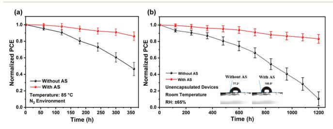
Fig. 4 Long-term stability of PSCs prepared without and with AS method at different ambient atmosphere without any encapsulation (a) 85 °C in N<sub>2</sub> environment; (b) 25 °C, 65%RH (the insert image showed the contact angle test of devices without and with AS method).
