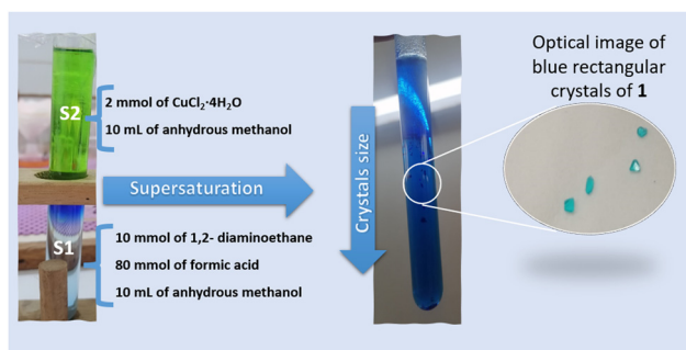
Fig. 1 Schematic representation of the synthesis of (NH 3 (CH 2 ) 2 NH 3 )[Cu(HCO 2 ) 4 ] single crystals using a facile slow diffusion process. The copper solution (S2) is gently added on top of a solution containing a mixture of organic linkers (S1). Blue crystals with different sizes are formed at the interface and at the bottom of the tube.
