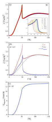
Fig. 8 (a) C/T vs. T curves of CoTeO<sub>4</sub> in the range  $0 \le H \le 12$  T. Inset in (a) represents the zoom view of peak maxima. (b) Magnetic (blue) and lattice (black) contributions of C/T vs. T for H = 0 T. (c)  $S_{\text{magnetic}}$  vs. T for H = 0 T.
