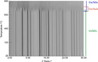
Fig. 5 Temperature-dependent SPXRD in situ study of CoTeO<sub>4</sub> using a wavelength of 0.4087 Å. The existence range of present phases is indicated on the right.
