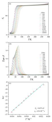
Fig. 10 (a)  $\varepsilon_r$  vs. T plots and (b) Tan  $\delta$  vs. T plots of CoTeO<sub>4</sub> crystal aggregates at selected frequencies and in zero magnetic field. (c)  $\ln \tau$  vs. 1/T plot; scattered symbols are the peak maxima of Tan  $\delta$  and the solid line is the least-squares straight line fit according to an Arrhenius equation.
