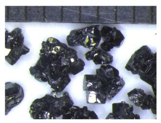
Fig. 2 Crystal aggregates of CoTeO<sub>4</sub>. The distance between the scale
