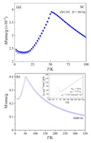
Fig. 9 (a) ZFC/FC *M vs. T* curves of CoTeO<sub>4</sub> for H=50 Oe; (b) M(T) under H=5 kOe. Inset in (b) shows  $(\chi-\chi_0)^{-1}$  vs. T and linear Curie–Weiss fit in the range  $70 \le T \le 300$  K. The obtained parameters are indicated in the Figure.
