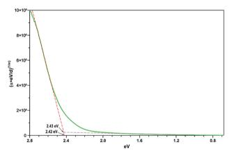
Fig. 14 Direct bandgap Tauc plot derived from the unpolarized transmission spectrum of CoTeO<sub>4</sub> using a crystal plate with a thickness of  $\sim$ 5  $\mu m$ .
