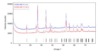
Fig. 1 X-ray powder diffraction patterns of single-phase CoTeO<sub>4</sub> tempered for 2 days at 550 °C and for 20 days at 600 °C. Tick marks represent the position of Bragg reflections.
