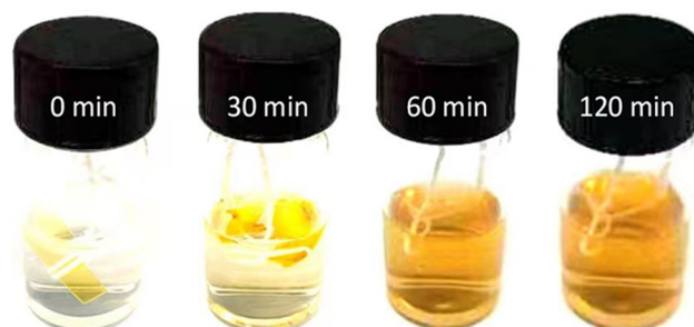
Fig. 9 Degradation process of VTCO-IPDI at different times in a 1 M HCl H 2 O/HFP (1/9, v/v) solution.
