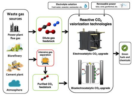
Fig. 1 Overview of emerging  $CO_2$  capture and conversion pathways. Proposed process flow for electrified  $CO_2$  conversion with selection of waste gas feedstock, omission or inclusion of gas separation device, and choice of  $CO_2$  conversion nanotechnology.
