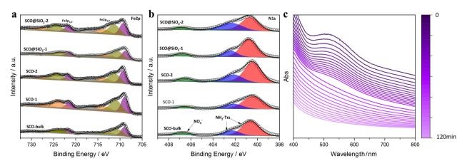
Fig. 2 Spectra from XPS of Fe 2p (a) and N 1s (b) of the different NPs and the bulk. (c) Dependency of the UV-vis absorbance of SCO@SiO<sub>2</sub>-1 redispersed in water as a function of time.
