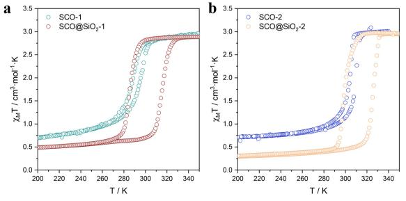
Fig. 3 Comparison of the thermal variation of the  $\chi_M T$  product for SCO-1 and SCO@SiO<sub>2</sub>-1 (a), and SCO-2 and SCO@SiO<sub>2</sub>-2 (b).
