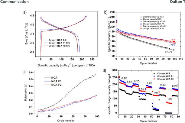
Fig. 3 Galvanostatic voltage profiles of NCA/Li, NCA-F1/Li, and NCA-F2/Li cells cycled at C/5 between 4.5 and 2.5 V versus Li<sup>+</sup>/Li; the first cycle is displayed (a); specific charge capacity of NCA/Li, NCA-F1/Li, and NCA-F2/Li cells cycled at C/5 (b); polarisation as a function of the cycle number for NCA, NCA-F1 and NCA-F2 cells (c); and current rate capability of NCA, NCA-F1, and NCA-F2 electrodes (d).
