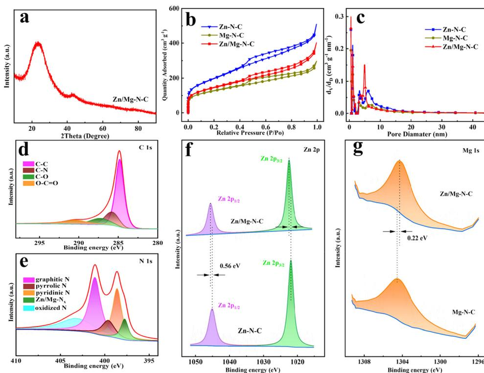
**Fig. 2** (a) XRD pattern of Zn/Mg-N-C. (b) Nitrogen adsorption/desorption isotherms and (c) pore size distribution curves of Zn/Mg-N-C, Zn-N-C and Mg-N-C. High-resolution XPS spectra of (d) C 1s and (e) N 1s of Zn/Mg-N-C. (f) Zn 2p XPS spectra of Zn/Mg-N-C and Zn-N-C. (g) Mg 1s XPS spectra of Zn/Mg-N-C and Mg-N-C.
