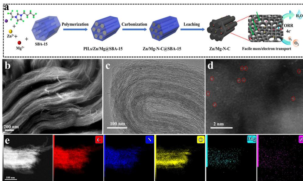
**Fig. 1** (a) Schematic diagram of the synthesis process of the Zn/Mg-N-C catalyst. (b) SEM and (c) TEM images of Zn/Mg-N-C. (d) HAADF-STEM image of Zn/Mg-N-C. (e) HAADF-STEM image of Zn/Mg-N-C and the corresponding elemental maps.
