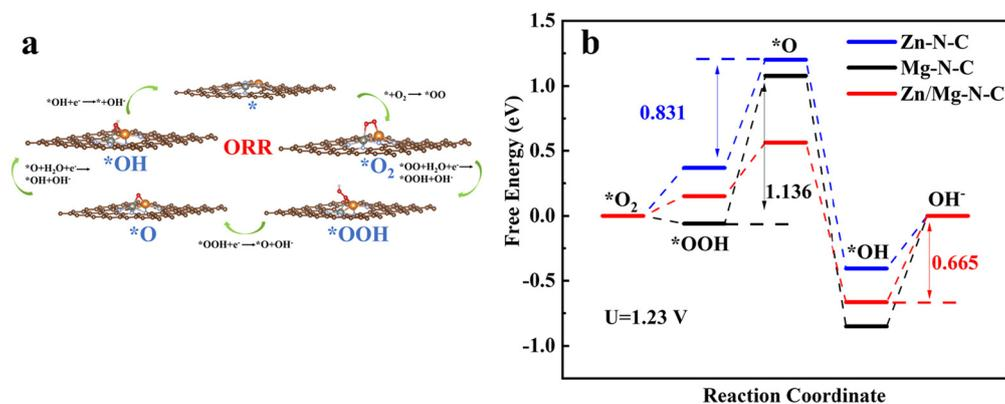
**Fig. 5** (a) The reaction pathway of the ORR by using Zn/Mg–N–C as an example. (b) The Gibbs free energy diagram of the ORR on Zn/Mg–N–C, Zn–N–C and Mg–N–C obtained from DFT calculations ( $U = 1.23$  V).
