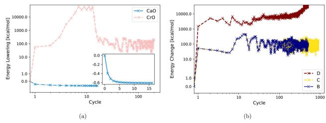
Energy change (zeroed at first iteration) during SCF cycles within DM21 for (a) CaO and CrO using Strategy A. (b) CrO using Strategy B, C, D.
