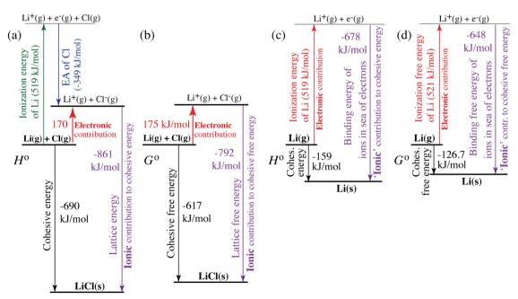
Fig. 4 Quantification of electronic (red, upwards) and ionic (purple, downwards) contributions to the cohesive energy of (a) and (b) LiCl(s) and (c) and (d) lithium metal. (a) and (c) Enthalpies; (b) and (d) free energies. The diagrams correspond to generalized Born-Haber cycles.
