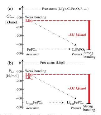
Fig. 2 Energetics and bonding of lithium in an iron phosphate-based lithium-ion battery. (a) Cohesive Gibbs free energy per atom. (b) Gibbs free energy per lithium atom, also known as the lithium (electro)chemical potential. The free-energy difference of  $-331 \text{ kJ mol}^{-1}$  between the reactants and the product can be released as electrical energy.
