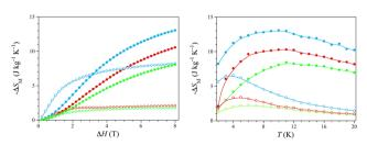
Fig. 3 Isothermal (left) and isofield (right) curves of the magnetic entropy change for **1** (red), **2** (green), and **3** (blue) at  $2 (\bigcirc)/10 \text{ K}$  ( $\bullet$ ) and  $2 (\bigcirc)/8 \text{ T}$  ( $\bullet$ ), respectively. The solid lines are only eye-guides.
