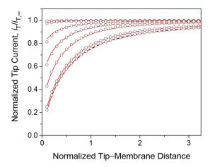
Fig. 3 Steady-state approach curves simulated for two-step (solid lines) and one-step (circles) transport with  $\kappa = 10$  and  $\rho = 1$ , and  $\lambda$  (=  $0.3\lambda_{mem}$ in eqn (25)) =  $10^2$ , 1,  $3 \times 10^{-1}$ ,  $1 \times 10^{-1}$ ,  $1 \times 10^{-2}$ , and  $1 \times 10^{-3}$  from the top to the bottom. Black dashed line represents an impermeable membrane
