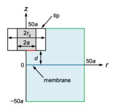
**Fig. 2** SECM diffusion problem of membrane transport in the cylindrical coordinate. The simulation space (light blue) is surrounded by eight boundaries (black, red, blue, and green lines). Boundary conditions at the tip and the membrane (red and blue lines, respectively) are given in the text. There is no normal flux at the symmetry axis and insulating surfaces (black lines). Simulation space limits are represented by green lines.
