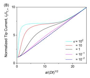
Fig. 6 Diffusion-limited chronoamperometric responses of two-step transport with  $\rho = 1$  as well as (A)  $\kappa = 10$  and various  $\lambda$  or (B)  $\lambda = 10^2$  and various  $\kappa$  at L = d/a = 0.1. Black dashed lines represent (A) an impermeable membrane and (B) diffusion-limited one-step transport with  $\lambda_{mem}$  =  $3.3 \times 10^3$  in eqn (25) with  $\lambda = 10^2$ ,  $\kappa = 10$ , and  $\rho = 1$ .
