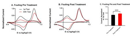
Fig. 7 Electrode fouling measurements at an untreated and a KOH treated CNTYME. 1  $\mu$ M 5-HT was injected for 5 seconds every 30 seconds, repeated 30 times. (A) CVs from an untreated CNTYME show a decrease on the 30th injection. (B) CVs from a 1-minute KOH treated CNTYME show the signal is largely preserved on the 30th injection. (C) Unpaired *t*-tests compare the 1st and 30th signal (p < 0.001, n = 4) and there was a significant difference in the fouling.
