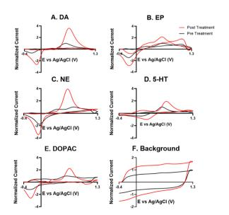
Fig. 5 FSCV results pre- and post-KOH treatment for a CNTYME. Measurements were collected on a CNTYME pre- (black) and post- (red) treatment for (A) 1  $\mu$ M DA, (B) 1  $\mu$ M EP, (C) 1  $\mu$ M NE, (D) 1  $\mu$ M 5-HT, (E) 20  $\mu$ M DOPAC, and for the (F) background.
