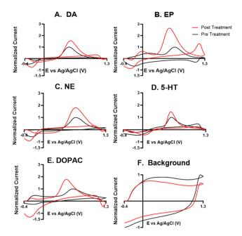
Fig. 3 FSCV results pre- and post-treatment for a CFME. Measurements were collected on a CFME pre- (black) and post- (red) treatment for (A) 1  $\mu$ M DA, (B) 1  $\mu$ M EP, (C) 1  $\mu$ M NE, (D) 1  $\mu$ M 5-HT, (E) 20  $\mu$ M DOPAC, and for the (F) background.
