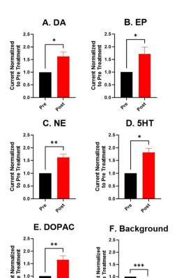
Fig. 4 Statistics on current pre- and post-KOH treatment for each neurotransmitter on a CFME. Paired t-tests were performed for each analyte, normalized to pre-treatment (1), n=6. (A) 1  $\mu\text{M}$  DA (p<0.05), (B) 1  $\mu\text{M}$  EP (p<0.05), (C) 1  $\mu\text{M}$  NE (p<0.01), (D) 1  $\mu\text{M}$  5-HT (p<0.05), (E) 20  $\mu\text{M}$  DOPAC (p<0.01), and (F) background (p<0.001).
