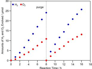
Fig. 6 Time course of water-splitting activity for the Pt<sub>NC</sub>/STO:Rh-BiVO<sub>4</sub> composite Z-scheme system using FeCl<sub>2</sub> as a mediator. Light source: a 300 W Xe lamp with a long-pass filter ( $> \sim 410$  nm), catalyst: 100 mg for each catalyst, reactant solution: 120 mL of 2 mmol  $L^{-1}$  FeCl<sub>2</sub> in  $H_2SO_4$  aq. (pH 2.4), reaction cell: a top-window reaction cell.
