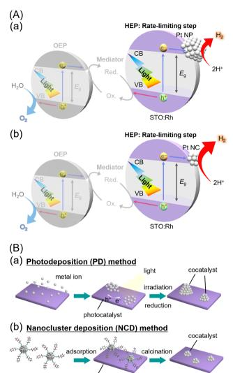
Fig. 1 Schematic illustrations of (A) Z-scheme photocatalytic water splitting and (B) the preparation procedure of cocatalysts on the photocatalysts using the (a) conventional PD method and (b) NCD method. In (A), CB, conduction band; VB, valence band;  $E_{q}$ , band gap; Red, reductants; and Ox, oxidants. STO:Rh is one of the most advanced HEP. The improvement in water-splitting activity can be expected by enhancing the reaction in HEPs, which is the rate-limiting step
