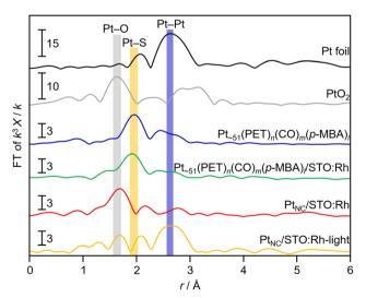
Fig. 2 Pt L3-edge FT-EXAFS spectra of  $Pt_{\sim 51}(PET)_n(CO)_m(p-MBA)_l$ , before  $(Pt_{\sim 51}(PET)_n(CO)_m(p-MBA)_l/STO:Rh)$  and after  $(Pt_{NC}/STO:Rh)$  calcination of Pt NC-loaded STO:Rh, and after light irradiation of Pt<sub>NC</sub>/STO:Rh (Pt<sub>NC</sub>/ STO:Rh-light). Pt foil and PtO<sub>2</sub> powder are also shown for comparison.
