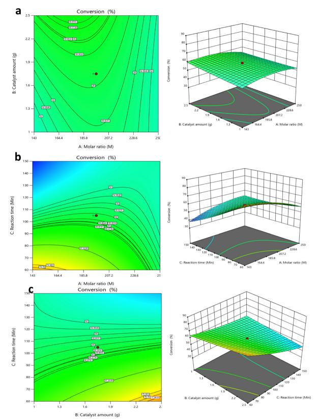
Fig. 10 Contour plot and 3D response curve for conversion of TS to FAME (biodiesel), (a) interaction of catalyst amount and molar ratio, (b) interaction between reaction time and molar ratio and (c) interaction between reaction time and catalyst amount.
