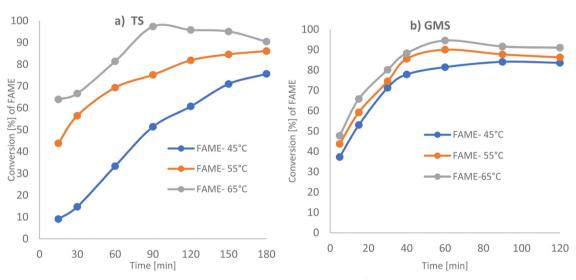
Fig. 5 GC-FID analysis for conversion of TS and GMS to FAME as a function of temperature (a) TS to methyl stearate for the molar ratio of methanol to TS 285.5:1, total vol. 108.95 mL, 6 g of PANF base catalyst; (b) GMS to methyl stearate for the molar ratio of methanol to GMS 115.1:1, total vol. 107.74 mL, 2.5 g of PANF base catalyst.
