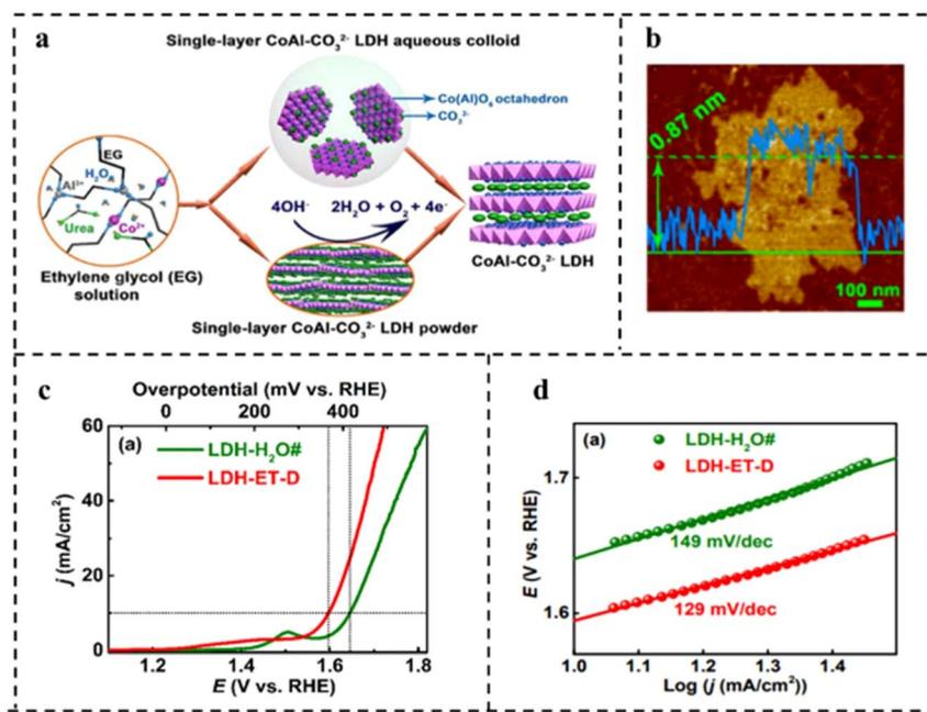
Fig. 14 (a) Schematic diagram of synthesis of water-dispersible single-layer  $\text{CoAl-CO}_3^{2-}$  LDH. (b) AFM image of single-layer  $\text{CoAl-CO}_3^{2-}$  LDH. (c) Polarization curves in  $\text{O}_2$ -saturated 1 M KOH at a scan rate of  $0.5 \text{ mV s}^{-1}$ . (d) Tafel plots corresponding to (c). Reproduced with permission from ref. 116. Copyright 2017, American Chemical Society.
