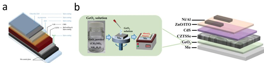
Fig. 4 (a) Schematic diagram of CZTS solar cells.<sup>43</sup> Reproduced with permission from ref. 43. (b) Schematic diagram of CZTSSe devices containing  $\text{GeO}_2$  layers.<sup>46</sup> Reproduced with permission from ref. 46.
