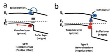
Fig. 5 Types of heterojunction interface alignments for the absorber and buffer layers: (a) type I (spike), (b) type II (cliff).<sup>33</sup> Reproduced with permission from ref. 33.
