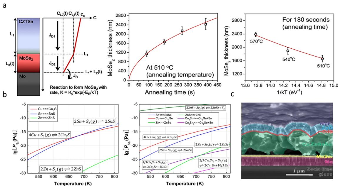
Fig. 1 (a) Schematic diagram of Se diffusion through CZTSSe/MoSe<sub>2</sub>/Mo during high-temperature annealing.<sup>48</sup> Reproduced with permission from ref. 48. (b) Equilibrium S vapor pressure vs. sulfuration temperature for the reactions and equilibrium Se vapor pressure vs. selenization temperature for the reactions.<sup>49</sup> Reproduced with permission from ref. 49. (c) Pinholes at the back interface of the CZTSSe solar cell.<sup>50</sup> Reproduced with permission from ref. 50.
