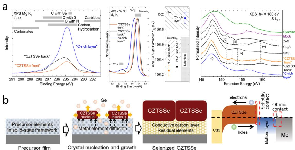
Fig. 3 (a) C 1s XPS, Se 3d XPS, and XES spectra of the investigated samples.<sup>64</sup> Reproduced with permission from ref. 64. (b) Schematic diagrams of the TGA-ammonia method and the energy-band structure of the cell.<sup>63</sup> Reproduced with permission from ref. 63.
