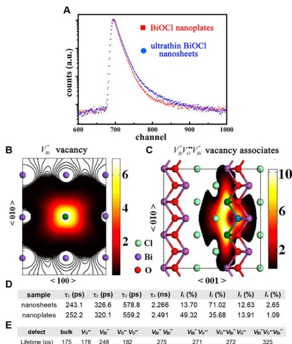
Fig. 8 (A) PAS spectra of ultrathin BiOCl nanosheets and nanoplates. (B and C) Schematic illustrations of trapped positrons of  $V_{\text{Bi}}$  defects and associated defects  $V_{\text{Bi}}^{\prime\prime}V_{\text{O}}^{\prime\prime}V_{\text{Bi}}^{\prime\prime}$ . (D) Positron lifetime parameters of ultrathin BiOCl nanosheets and nanoplates. (E) Calculated positron lifetime values of BiOCl.<sup>104</sup> Copyright © 2013 American Chemical Society.
