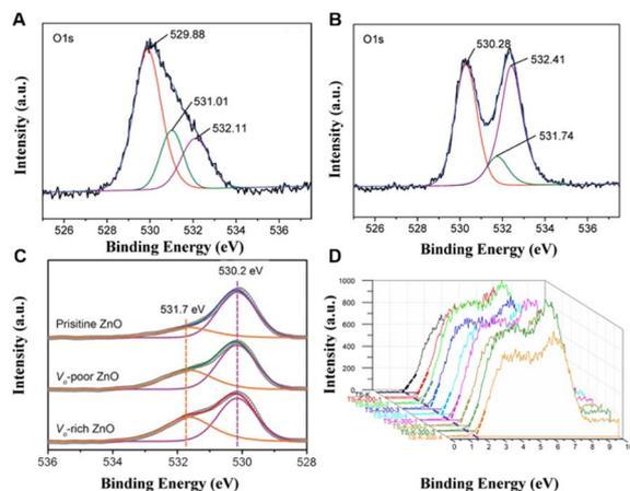
Fig. 10 (A) XPS of pure TiO<sub>2</sub> nanorods and (B) TiO<sub>2</sub> nanorods with Cu doping.<sup>110</sup> Copyright © 2010 American Chemical Society. (C) XPS of V<sub>O</sub>-rich ZnO.<sup>112</sup> Copyright © 2012 American Chemical Society. (D) XPS valence band spectra of black TiO<sub>2</sub> samples.<sup>113</sup> Copyright © 2018 Elsevier Inc.
