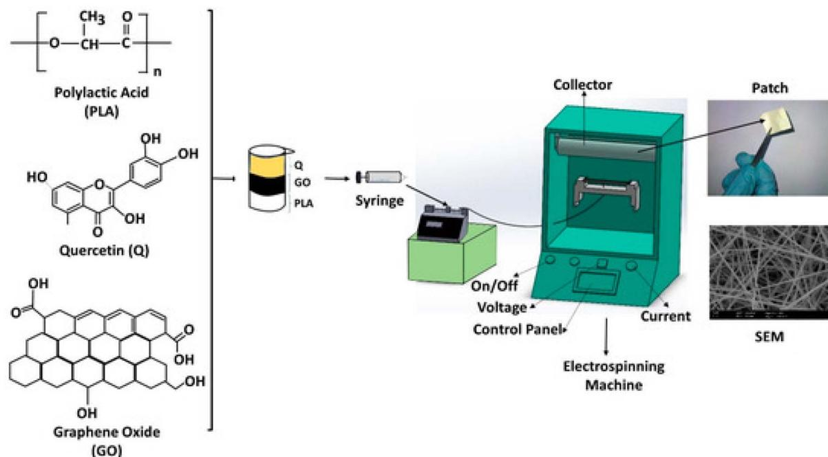
Fig. 11 Fabrication of PLA/GO/Q by electrospinning.<sup>92</sup>
