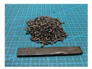
Fig. 18 100% natural biomass biodegradable thermoplastic material made from wood, stone and natural deep eutectic solvent.<sup>86</sup>
