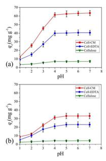
Fig. 15 Adsorption efficiencies of extracted cellulose, cell-EDTA (ethylene diamine tetra acetic acid-modified nanocellulose), and cell-CM (carboxy methyl group-modified nanocellulose) for (a) Pb<sup>2+</sup> and (b) Cd<sup>2+</sup> in the pH range of 1–7. Conditions for adsorption: concentration of  $Pb^{2+}$  or  $Cd^{2+} = 100 \text{ mg L}^{-1}$ , at room temperature for 90 min.81
