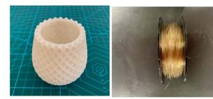
Fig. 38 Cellulose-based biomass biodegradable resin mold product made by 3D printer and resin filament for 3D printer.
