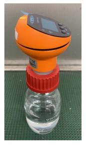
Fig. 3 Commercial biodegradability measuring machine.
