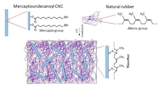
Fig. 32 Illustration of the thiolene coupling reaction between natural rubber and modified cellulose nanocellulose in nanocomposite. 156
