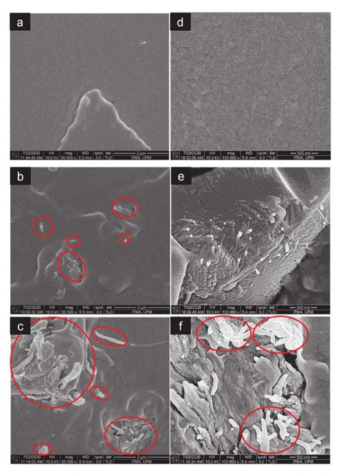
Fig. 12 FESEM images at  $500\,00\times$  and  $1\,000\,00\times$  magnification of the fractured surfaces of neat PLA (a and d), PLA/CNF3 (b and e), and PLA/CNF6 (c and f), respectively. Red circles show nanocellulose. PLA/CNF6 exhibits agglomerated nanocellulose. CNF: nanocellulose. Number after CNF indicates the % against the weight of PLA.<sup>60</sup>
