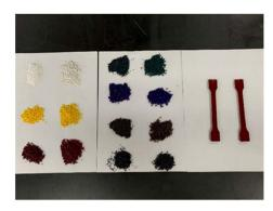
Fig. 23 Biomass biodegradable color masterbatch.
