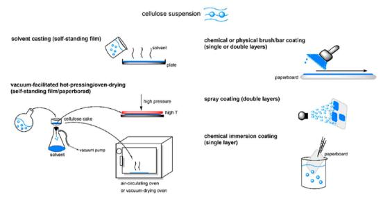
Fig. 8 Procedure for the preparation of cellulose-based bioplastic by casting method.<sup>55</sup>
