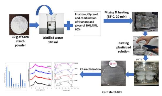
Fig. 6 Procedure for the preparation of starch-based bioplastic by the casting method.<sup>51</sup> Starch bioplastic was prepared by mixing corn starch, water and plasticizer.
