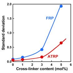
Fig. 5 The effect of the cross-linker content on the standard deviation of  $\langle l \rangle_T$  for the ATRP (red) and FRP (blue) gels at 25 °C.
