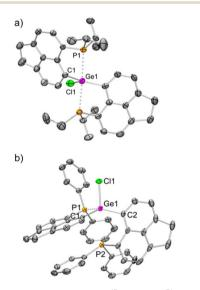
Fig. 2 (a) Molecular structures of (a)  $2^{iPr}$  and (b)  $2^{Ph}$  (H atoms, solvent molecule and triflate anion have been removed for clarity; thermal ellipsoid 50%). Selected bond lengths [Å] and angles [°]: (a) Ge1-Cl1=2.228(2), Ge1-Cl=1.988(4), Ge1-Pl=2.643(1); Cl-Ge1-Cl=1.47.9(2), Cl1-Ge1-Cl=1.06.1(1), Cl1-Ge1-Pl=86.9(1), Pl-Ge1-Pl=1.73.9(1); (b) Ge1-Cl=1.922(3), Ge1-Cl=1.926(3), Ge1-C
