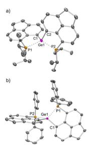
Fig. 3 Molecular structures of (a)  $3^{iPr}$  and (b)  $3^{Ph}$  (H atoms, solvent molecules and triflate anions have been removed for clarity; thermal ellipsoid 50%). Selected bond lengths [Å] and angles [°]: (a) Ge1-C1=1.923(5), Ge1-C2=1.923(5), Ge1-P1=2.350(1), Ge1-P2=2.363(1); C1-Ge1-C2=112.5(2), P1-Ge1-P2=122.4(1), C1-Ge1-P1=90.9(2), C2-Ge1-P2=91.4(2), C1-Ge1-P2=120.8(2), C2-Ge1-P1=121.2(2); (b) Ge1-C1=1.924(3), Ge1-C2=1.920(3), Ge1-C2=1
