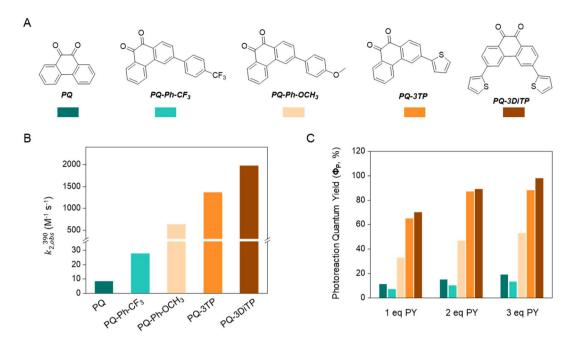
Fig. 2 Overview of the second order reaction rate ( $k_2$ ) and photoreaction quantum yield ( $\Phi_P$ ) of the PQ-ERA photoclick reaction system. (A) Structures of the investigated PQs, (B)  $k_2$  obs. (390) and (C)  $\Phi_P$  of PQ-ERA photoclick reaction.
