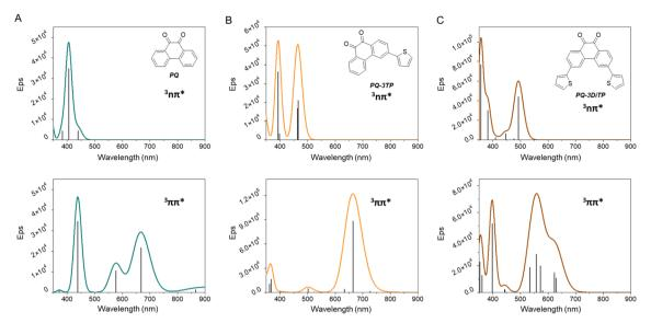
Fig. 6 Calculated absorption spectra for the  $^3n\pi^*$  (up) to  $^3\pi\pi^*$  (down) states of (A) PQ, (B) PQ-3TP and, (C) PQ-3DiTP. Stick spectra have been convoluted with a Gaussian profile with a width of 0.1 eV for further comparison with the experiment.
