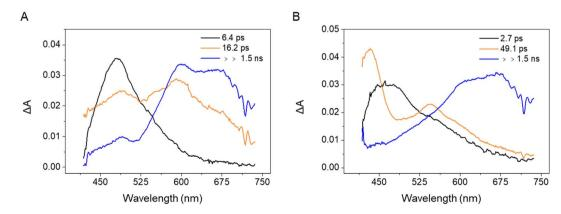
Fig. 4 EADS obtained from a global analysis of the transient absorption data recorded for (A) PQ-3TP and (B) PQ-3DiTP in MeCN upon excitation at 400 nm.
