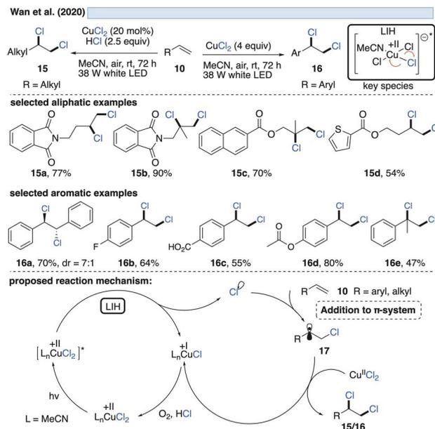
Scheme 5 Vicinal dichlorination of activated and unactivated olefins.
