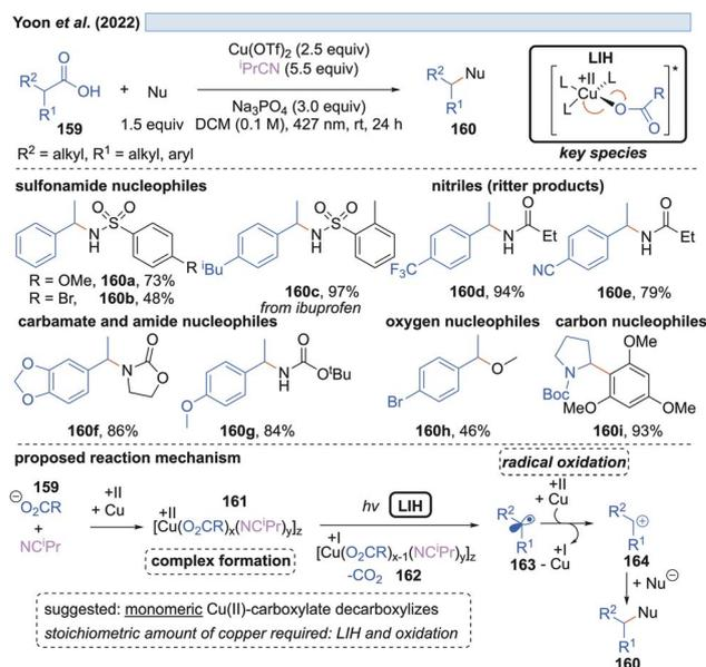
Scheme 24 Decarboxylative cross-coupling reaction with different nucleophiles.
