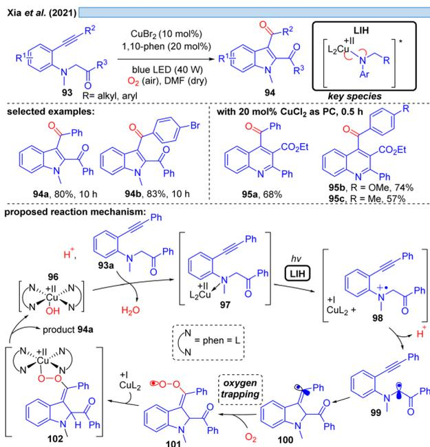
Scheme 15 Cu(II)-photocatalyzed oxidative cyclization reaction of aromatic amines.
