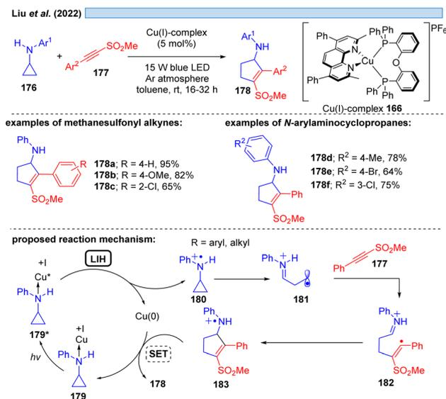
Scheme 26 Copper-catalyzed [3 + 2] cycloaddition involving a Cu(I)\* / Cu(0) cycle.
