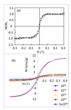
Fig. 9 (a) Magnetization (M) *versus* applied field (H) curves for the detonation NDs (d=4-5 nm) ( $M_s=$  saturation magnetization) with  $^{15}$ N dose at (a)  $5\times 10^{14}$  cm $^{-2}$  and (b) various doses: enhanced magnetizations were observed with doses above  $5\times 10^{16}$  cm $^{-2}$ .<sup>144</sup> Reproduced with permission from ref. 144 Copyright 2005 American Physical Society.
