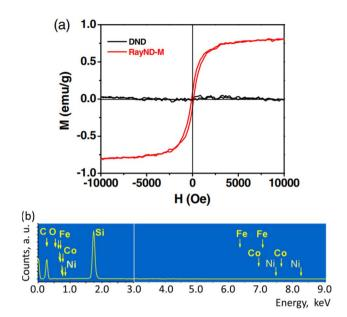
Fig. 10 Magnetic properties of RayND-M (d=4.3-4.5 nm). (a) Magnetization curve of RayND-M [in comparison with ordinary detonation ND (DND), d=3-10 nm]. (b) EDS spectrum of RayND-M; Fe, Co, and Ni atoms as impurities were not detected. Reproduced with permission from ref. 139 Copyright 2018 SPIE.
