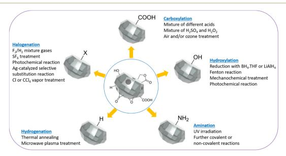
Fig. 2 Schematic representation of homogenization of ND surfaces via carboxylation, hydroxylation, hydrogenation, amination, and halogenation.87
