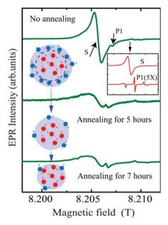
Fig. 8 EPR analysis of 50 nm NDs before and after air annealing for 5 and 7 h. The inset on the top right shows contributions of nitrogen impurity centers (labeled as P1) and surface spins (labeled as S) to the EPR spectra. The EPR spectra under the annealing process are shown below. The red dots in the drawing represent the P1 centers and the blue dots represent surface spins. 143 Reproduced with permission from ref. 143 Copyright 2020 American Institute of Physics.
