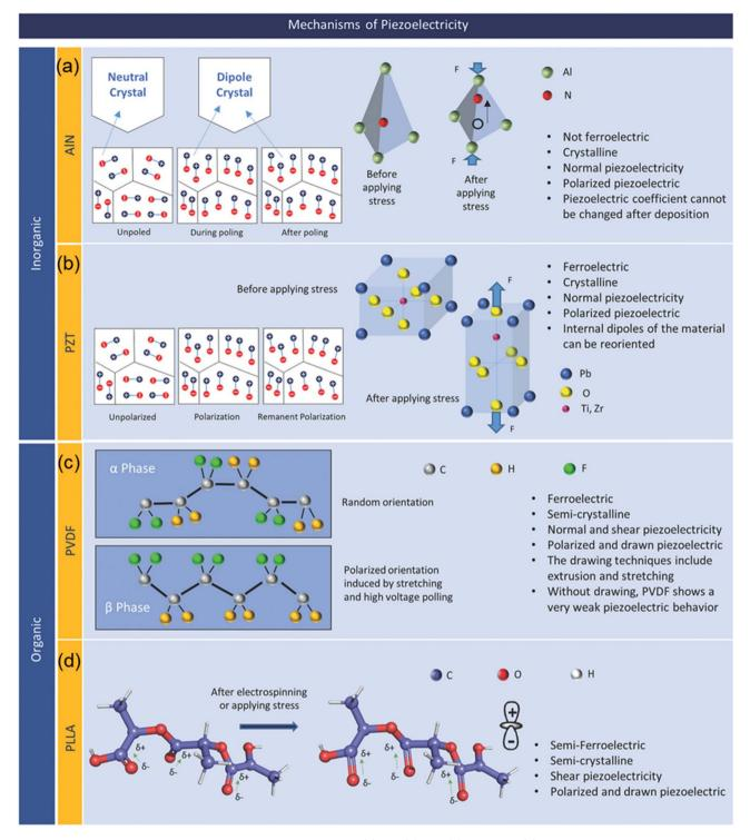
Fig. 2 Representative piezoelectric materials and their mechanisms: (a) AlN; (b) PZT; (c) PVDF; and (d) PLLA. Reproduced with permission from ref. 32 Copyright 2019 John Wiley and Sons.
