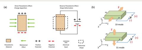
Fig. 1 Schematic illustration of (a) electromechanical conversion process by the piezoelectric effect (reproduced with permission from ref. 31 Copyright 2021 Elsevier), and (b) operation modes of the piezoelectric effect (reproduced with permission from ref. 30 Copyright 2018 AIP Publishing).
