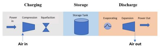
Fig. 2 LAES cycle principle of work.
