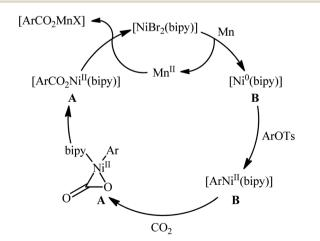
Scheme 26 Mechanistic proposal for the formation of carboxylic acid derivatives 46.
