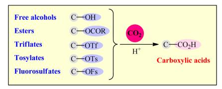
Fig. 1 Reductive carboxylation of C-O bonds with CO<sub>2</sub>.
