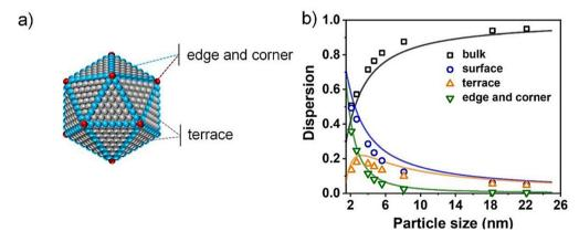
Fig. 4 (a) Schematic diagram of a structurally stable icosahedral Pd NP. (b) The ratio of bulk, surface, terrace, edge, and corner atoms on icosahedral Pd NPs with different sizes. 72 Copyright 2020, the Royal Society of Chemistry.
