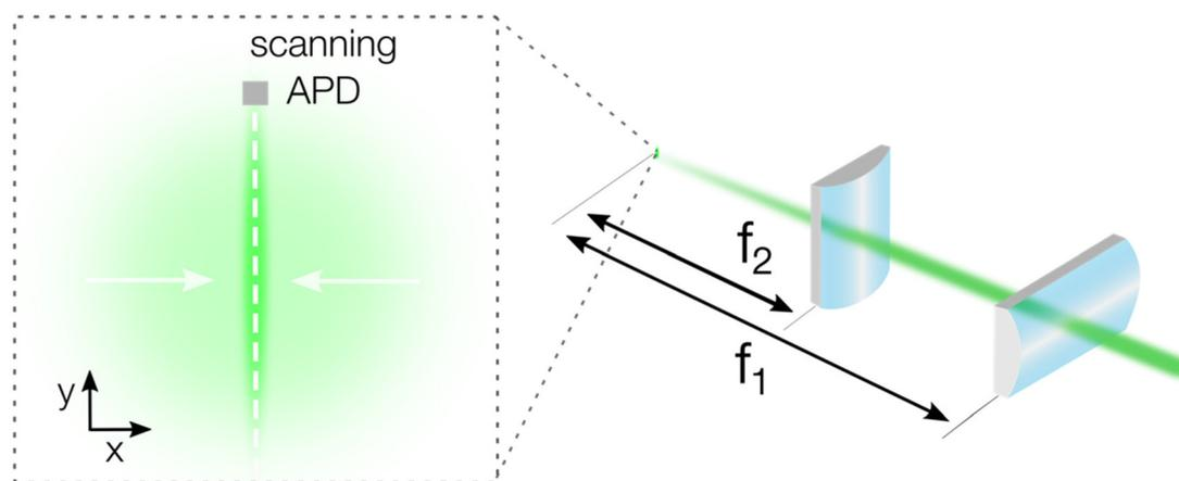
**Fig. 1** Set of cylindrical lenses placed along the light path towards the APD. The lenses highly magnify the PL emission spot along the scanning direction ( $y$ -axis) while simultaneously demagnifying it along the orthogonal direction ( $x$ -axis). The APD scan of the imaged PL spot is performed along the  $y$ -axis (white dashed line).
