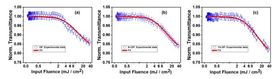
Fig. 8 Optical limiting onset curves of (a) DP, (b) Er-DP, and (c) Yb-DP. Open circular symbols represent experimental data and solid lines show theoretical fits.
