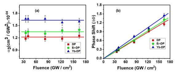
Fig. 7 Excitation-fluence dependences of (a) the three-photon absorption coefficient obtained from OA measurements and (b) the phase shift obtained from CA measurements. Scattered symbols represent experimental data while the solid lines are linear fits.
