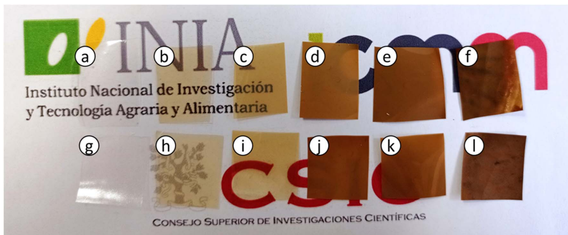
Fig. 2 Appearance of the bionanocomposite films: (a) HPMC, (b) H-0.5L, (c) H-1L, (d) H-3L, (e) H-5L, (f) H-10L, (g) H-3M, (h) H-3M-0.5L, (i) H-3M-1L, (j) H-3M-3L, (k) H-3M-5L, (l) H-3M-10L.
