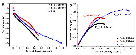
Fig. 7 (a) Polarisation and (b) power density curves obtained for Fe<sub>1</sub>Co<sub>1</sub>-ZNT-900, Fe<sub>1</sub>Co<sub>2</sub>-ZNT-900, and Pt/C cathode catalysts in H<sub>2</sub>/O<sub>2</sub> AEMFCs [anode catalyst: PtRu/C. AEM: Aemion+® 15  $\mu$ m. T = 65 °C].
