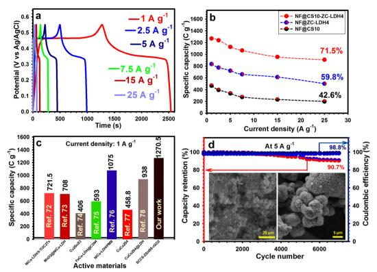
Fig. 6 (a) GCD profiles for the NF@CS10-ZC-LDH4 electrode from 1 to 25 A g<sup>-1</sup>. (b) Specific capacities vs. current densities for the NF@CS10, NF@ZC-LDH4, and NF@CS10-ZC-LDH4 electrodes. (c) Comparison of capacity values for NF@CS10-ZC-LDH4 with previously published values. (d) Longevity and coulombic efficiency of NF@CS10-ZC-LDH4 at 5 A g<sup>-1</sup> (the inset shows FE-SEM images of NF@CS10-ZC-LDH4 after 7000 cycles).
