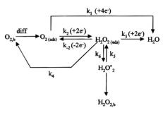
Fig. 1 Schematic diagram of the ORR process under acid conditions. 16
