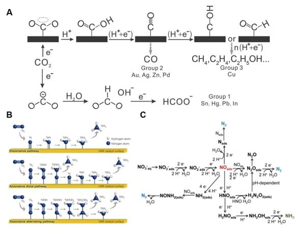
Fig. 2 (A) The possible pathways of multi-step activation and transformation of CO2 to various value-added products. Reprinted with permission from ref. 15. Copyright 2016, John Wiley & Sons, Inc.; Proposed roadmap of multi-step electroreduction of (B)  $N_2$  and (C)  $NO_3^-$  towards  $NH_3$ synthesis. Reprinted with permission from ref. 22 and 23. Copyright 2019, Elsevier and Copyright 2021, the Royal Society of Chemistry.
