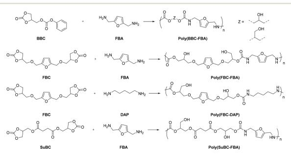
Fig. 31 Synthesis of main-chain furan-containing NIPUs by utilizing furan-based bis(cyclic carbonate) and diamine. Reaction conditions: DMF, 70 °C, up to 48 h.
