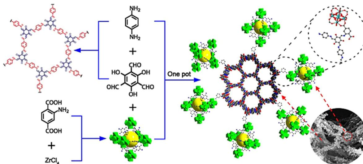
Fig. 19 Schematic illustration for designing an  $\text{NH}_2\text{-UiO-66/TpPa-1-COF}$  hybrid material. Adapted with permission, copyright, 2018, Wiley-VCH.<sup>124</sup>
