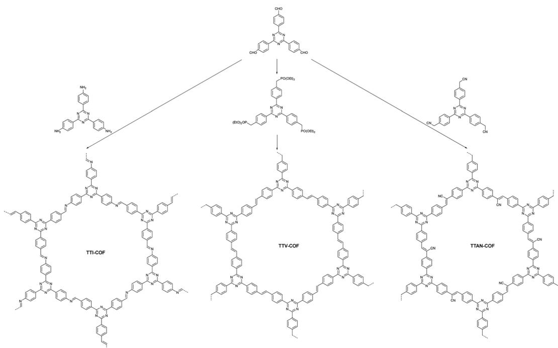
**Fig. 13** The synthesis processes of three COFs with different linkages.<sup>96</sup>
