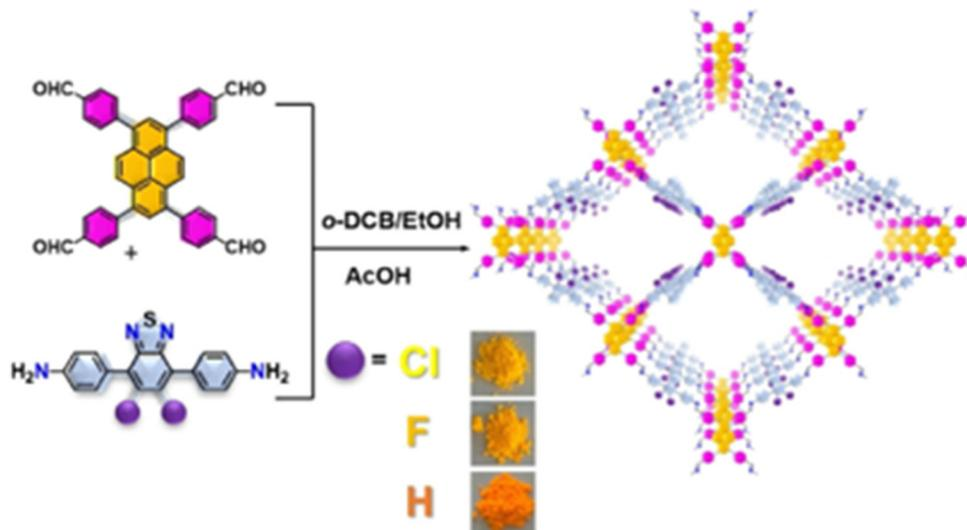
Fig. 6 Synthesis route and chemical structure of Py-XTP-BT-COF. Reprinted with permission, copyright, 2020, Wiley-VCH.<sup>70</sup>
