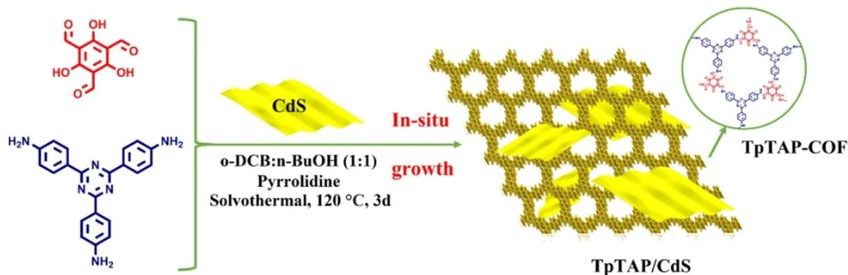
Fig. 17 Schematic illustration for constructing direct Z-scheme TpTAP/CdS. Adapted with permission, copyright, 2023, Elsevier.<sup>120</sup>
