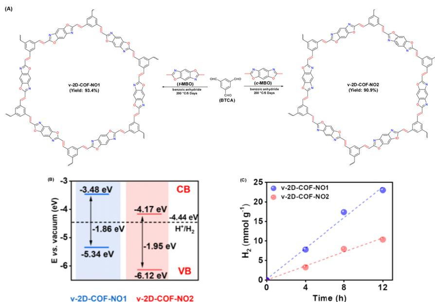
Fig. 12 (A) Schematic illustration for establishing v-2D-COF-NO1 and v-2D-COF-NO2. (B) Energy band position of v-2D-COFNO1 and v-2D-COF-NO2. (C) Time course of photocatalytic H<sub>2</sub> production activity for v-2D-COFNO1 and v-2D-COF-NO2. Reproduced with permission, copyright, 2022, American Chemical Society.<sup>94</sup>
