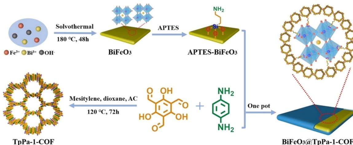
Fig. 18 Schematic illustration for fabricating a BiFeO<sub>3</sub>@TpPa-1-COF core-shell Z-scheme heterojunction hybrid. Adapted with permission, copyright, 2022, Wiley-VCH.<sup>123</sup>
