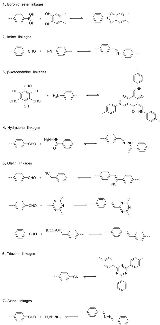
Fig. 1 Linkage chemistry for COF-based photocatalytic hydrogen production.
