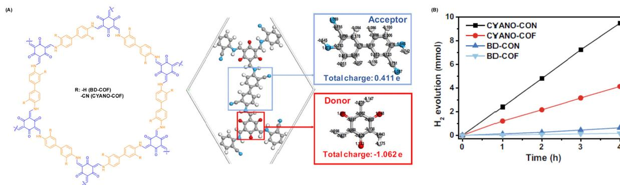
Fig. 7 (A) Structure diagram and charge distribution of CYANO-COF. (B) Time course of the photocatalytic H<sub>2</sub> evolution performance of different COFs and CONs. Reprinted with permission, copyright, 2022, Nature Publishing Group.<sup>69</sup>
