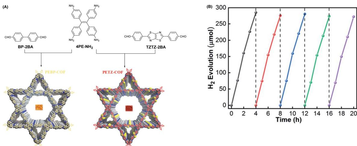
**Fig. 3** (A) Schematic description showing the fabrication of PEBP-COF and PETZ-COF. (B) Testing the cycling stability of PETZ-COF hydrogen precipitation for more than 20 h. Reprinted with permission, copyright, 2022, Royal Society of Chemistry.<sup>53</sup>
