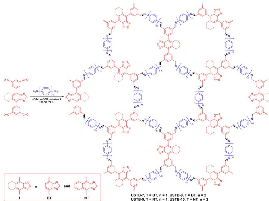
Fig. 8 Schematic diagram for synthesizing USBT-7 to USBT-10.<sup>81</sup>
