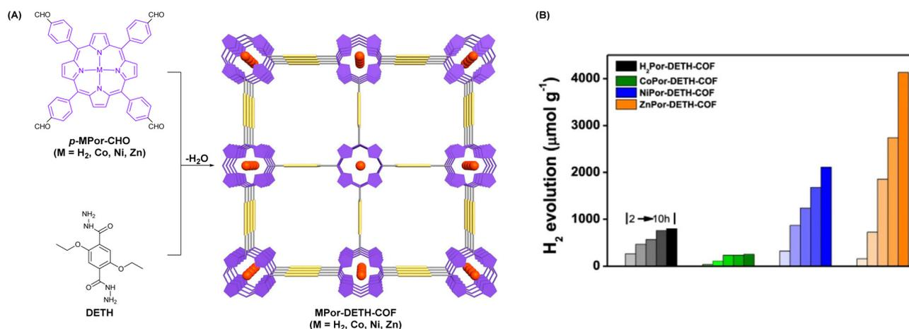
Fig. 16 (A) Schematic illustration for synthesizing MPor-DEPH-COF. (B) Time-dependent photocatalytic  $\text{H}_2$  evolution activity of MPor-DEPH-COF. Adapted with permission, copyright, 2021, Nature Publishing Group.<sup>105</sup>
